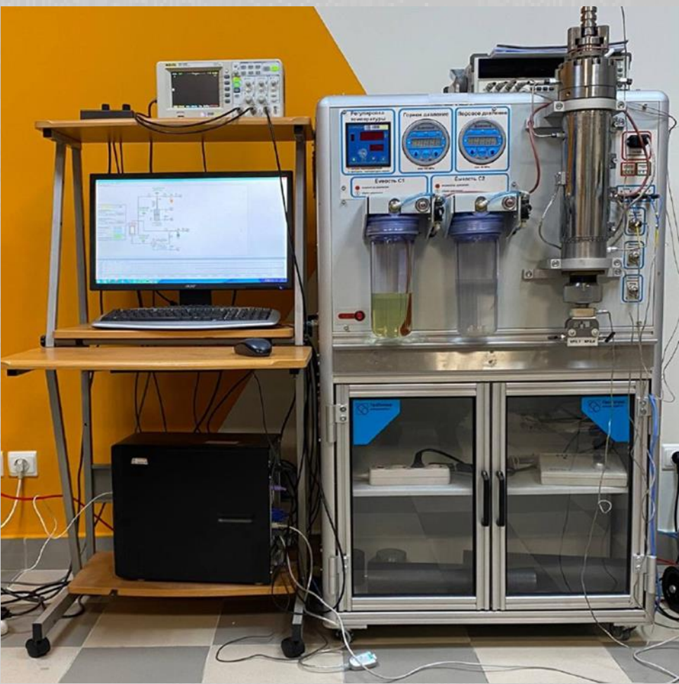
Fig. 2– Acoustic Property Measurement System «PIK-US-EP» (Geologika JSC, Novosibirsk)
